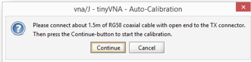
Please attach a RG-58 coaxial cable to the TX connector and click
