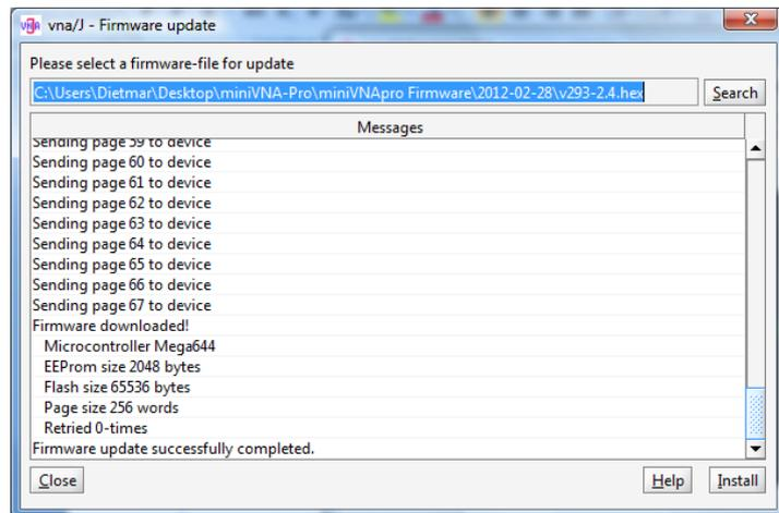
**Remark:** You can also use this procedure to downgrade to a previous firmware release!
