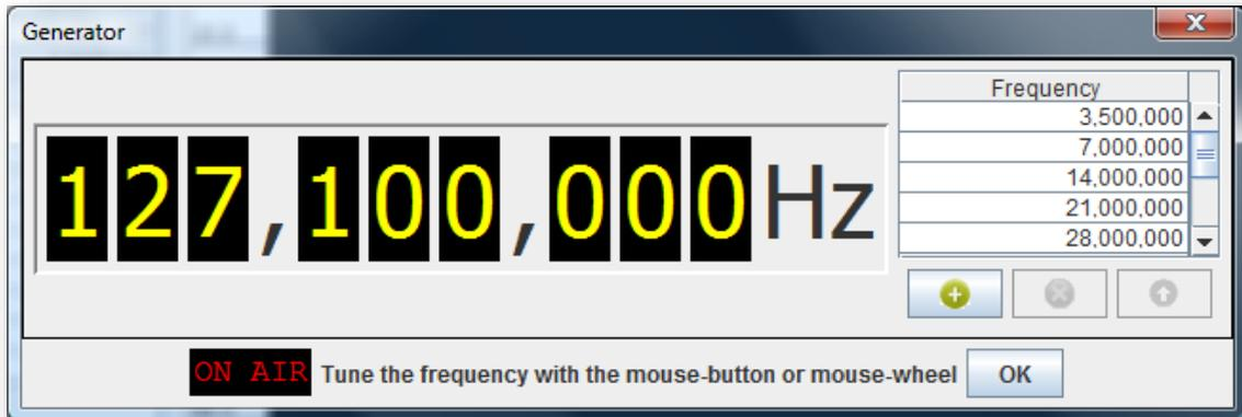
The frequency range is determined by the loaded driver. Details can be viewed in the driver info dialog.
