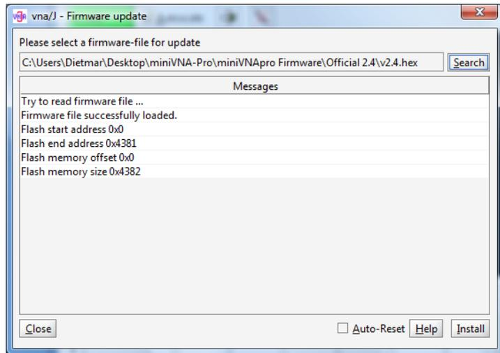
Select the “Install” button and the download of the firmware starts after the soft-reset of the miniVNA<sup>pro</sup>.
